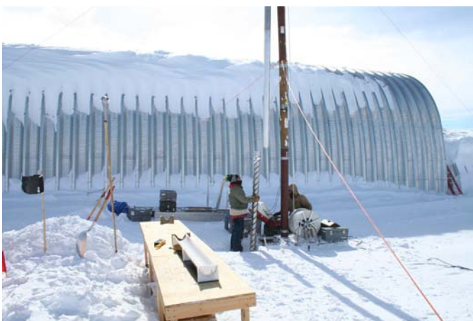
Bella Bergeron (left) and Michael Jayred (right), from ICDS, drill the 130 meter ice core. The tall arch in the background of the photo is the structure that will house the DISC Drill next year. The smaller arch on the right is the core-processing arch. Photo: J. Souney
