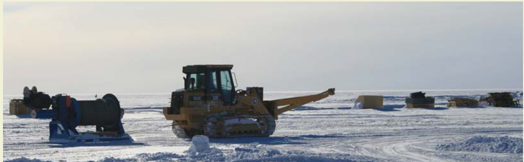
Moving the winch drum for the DISC Drill out to the arch facility. Photo: Dave Ferris (SDSU, 2007)
