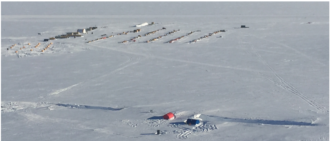
2016-17 WAIS Camp viewed from grid South. The drilling arch is in the foreground, invisible under the snow surface, accessed by 2 snow ramps. The red and blue logging support tents are on the surface outside the arch. In the background are the town line of camp, tent city, 5 cargo lines, the fuel bladders and skiway. Photo courtesy K. Webster
