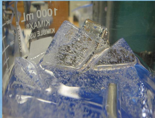
Ice melting under vacuum. Once released, the composition of the old air is measured with a mass spectrometer.
