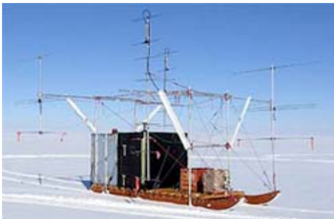
Fig. 2: Dual-frequency radar system on a 16-foot-long Komotek sled. The gray Faraday cage houses the radar system. The front black part hosts an operator during the polarimetric measurements. Bigger 8-element Yagi antennas are for 179 MHz, while smaller 3-element Yagi antennas are for 60 MHz. Transmitting and receiving antennas were installed at each side parallel to the sled axis so that the polarization-plane azimuth is consistent with that of the sled axis. As the shape of the antenna structure suggests Frankenstein, the sled was named Frankensled.
