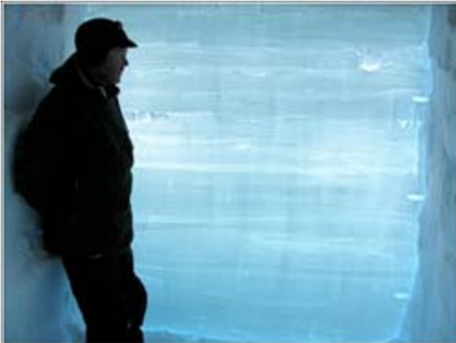
Fig. 1: A 2 meter backlit snowpit at WAIS Divide. Bright sections on right are 50cm intervals. The snowpit is at the exact location where the deep ice core will be drilled. The snowpit was sampled for chemistry, isotopes, density, and stratigraphy to 3 meters (after sampling the pit was then converted to a 2 meter backlit pit). The snowpit had to be done before construction of the arch facility, which will house the drill, could start at the site.
